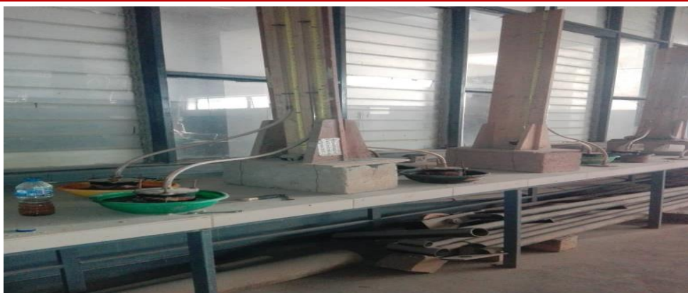
Plate 1: Hydraulic conductivity apparatus used for the test.
